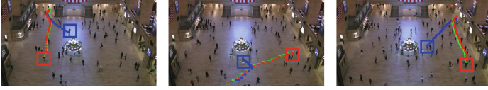
Fig. 9. Improved pedestrian tracking results by Behavior-CNN (red dots) and RFT [45] (blue dots). Ground truth trajectories are shown as green dots. Successfully tracked pedestrians of the proposed method and mis-tracked pedestrians by the RFT method are marked by the red and blue rectangles. (Color figure online)
