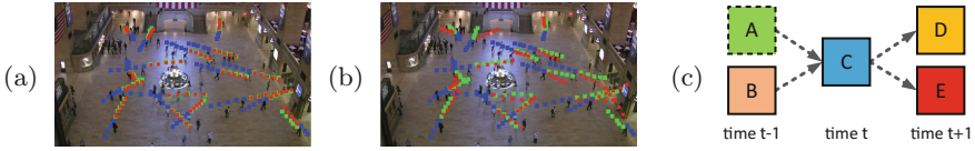
Fig. 1. Prediction results by the proposed Behavior-CNN (a) and the Social Force Model [15] (b). The input, predicted and ground-truth walking paths are shown as blue, red, and green dots, respectively. Only some pedestrians’ prediction results are shown in the figure. (c) Illustration of association ambiguity in dense flow maps. (Color figure online)
