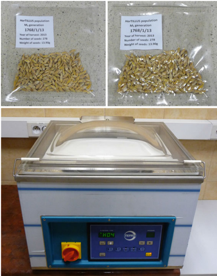
Fig. 6.2 Vacuum packer and seeds prepared for storage in a seed bank
