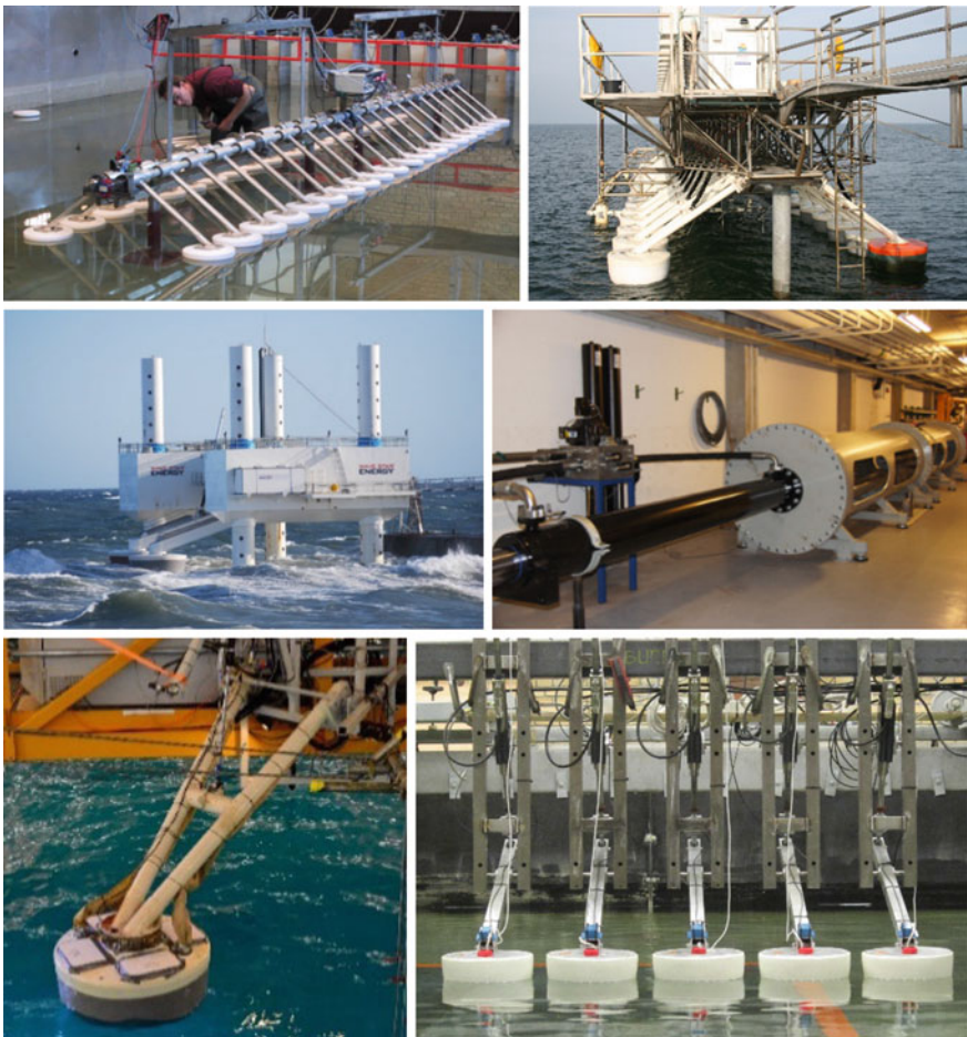
Fig. 9.2 Some of the development efforts behind the Wavestar WEC; top row an early stage lab model (TRL 2), a benign site prototype (TRL 5); second row a sea trial prototype (TRL 7) and a hydraulic PTO test bench; bottom row a large single float lab model and a lab model with advanced PTOs. Courtesy of Wavestar
