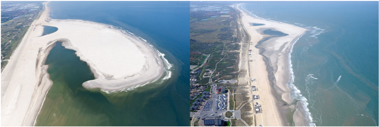
Fig. 18.3 Mega-nourishment ‘Delfland Sand Motor’. After completion in July 2011 ( left ) and in May 2015 ( right ) after reshaping ( https://beeldbank.rws.nl , Rijkswaterstaat/Joop van Houdt)
