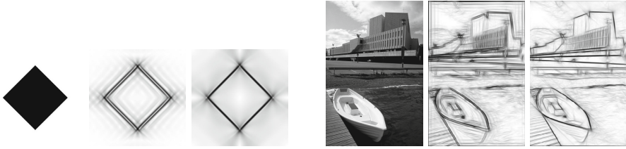
Fig. 2. Enhancement of signal discontinuities provided by Shearlets: two example images and the results obtained by choosing the \hat{\psi}_1 as the Lemarie-Meyer wavelet (center) or the Mallat wavelet (right).
