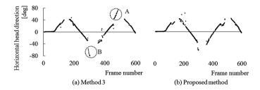
Fig. 7. Time course of detected horizontal head direction when subject rotates head in horizontal
