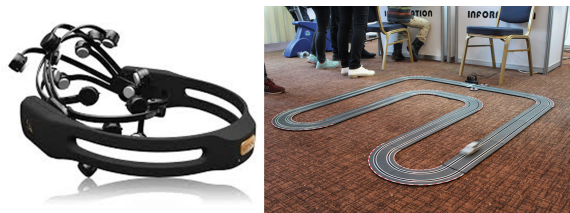
Fig. 2. EPOC and Carrera Slot Car (EPOC is as a 14-channel wireless EEG system developed by Emotiv Systems.)
