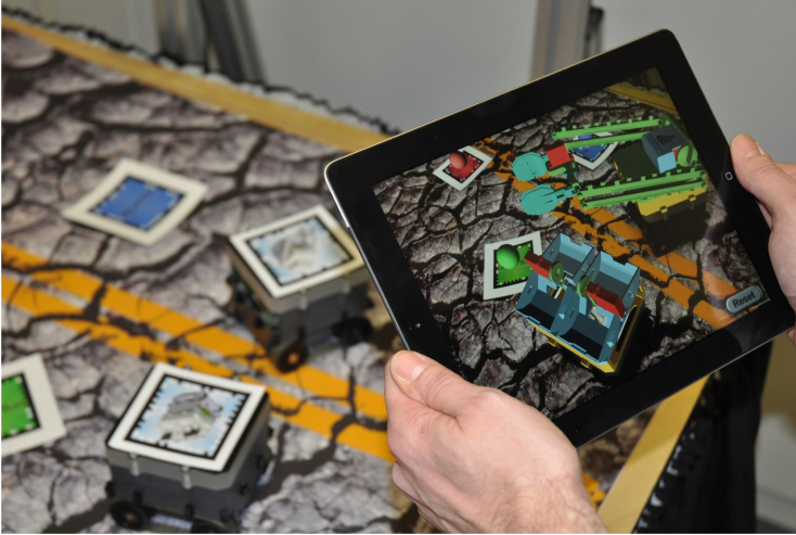
Fig. 1. Visualization of virtual modules on real BeBots using augmented reality.
