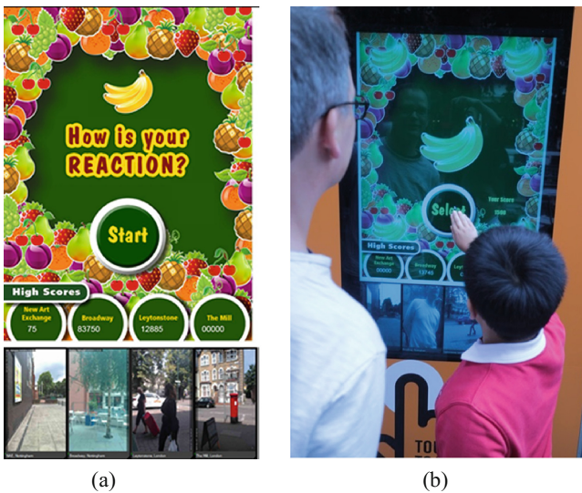
Fig. 2. Design of attention grabber game (a) Final home page layout with high scores and webcam feeds at bottom (b) Example of game play on the touchscreen.
