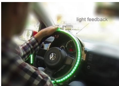
Fig. 3. The light feedback (color figure online)
