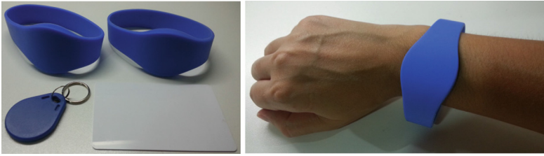
Fig. 2. Accessories that can be used for patient's identification, containing RFID tags: bracelets, card and keychain.
