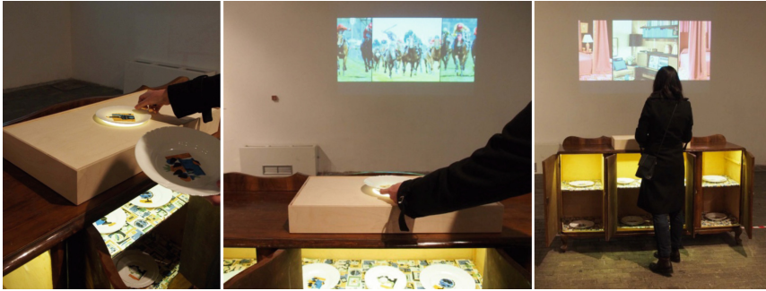
Fig. 2. Visitors may take a plate from the cabinet and place it on top (on the luminous circle) thus initiating a coherent triptych visual, relating to the dish image. The QR tags at the back of each plate, detected via the webcam and a PC, trigger the projection of related content.
