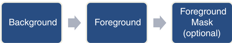
Fig. 2. Rendering order of different application layers: Background contains the pictures of the background sceneries, Foreground refers to the picture of the users and Foreground Mask includes all the parts of the background that appear in front of the users
