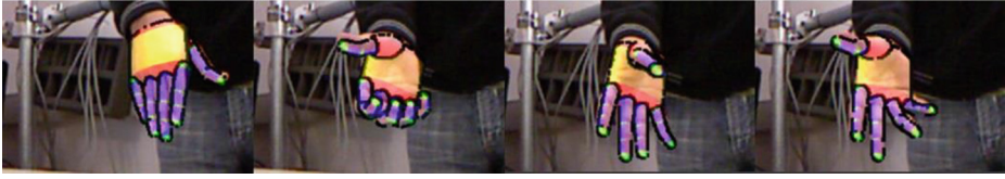
Fig. 3. Snapshots from a hand tracking sequence from [12], the hand model in the hypothesized solution is placed upon the real hand RGB image taken by Kinect® (Color figure online).
