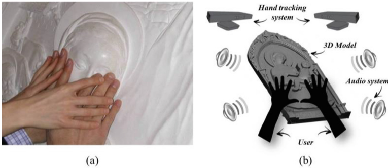
Fig. 2. (a) Typical exploration of artworks where skilled persons guide the hands of blind people [11] – (b) Conceptual framework of the exploration performed by the supposed system.
