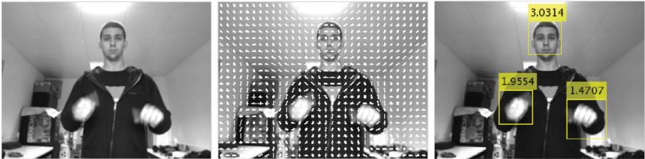
Fig. 3. (Left to right) a person in front of the robot in gray scale (left) coded by HOG-like features (middle) with detected face and hands (right).
