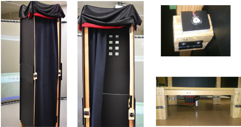
Fig. 6. Locker-like box and its attachments (photodiode sensor (top right), subwoofer speaker (bottom right))
