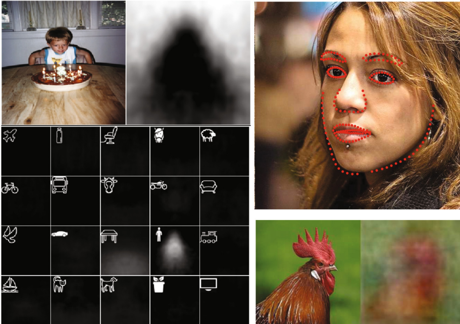
Fig. 1. How many different local image properties can be predicted from a generic ConvNet representation using a linear model? In this figure, given the ConvNet representation of an image, we have estimated three different local properties. Namely, semantic segmentation for background (top left) and 20 object classes (bottom left) present in PASCAL VOC dataset, 194 facial landmarks (top right) and RGB reconstruction of the original image (bottom right). One can see that a generic ConvNet representation optimized for ImageNet semantic classification has embedded high level of local information.
