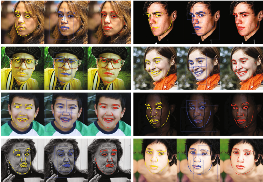
Fig. 3. The landmarks predicted by our linear regressors for eight different images from the Helen Dataset. The leftmost image in each triplet shows the ground truth. The middle image shows the landmarks predicted by the linear regression functions from the ConvNet representation of the whole image to landmark coordinates. In the middle image the bounding boxes, defined by the initial predictions for the landmarks, used by look-back method are also shown. The rightmost image shows the final landmark predictions made by the look-back method.
