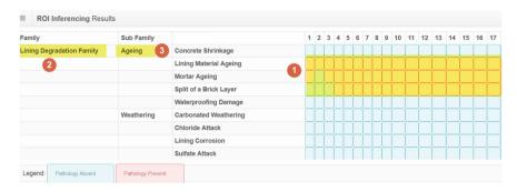
**Fig. 11.** The PADTUN interface showing the overview of pathologies across tunnel portions. (1) shows the regions of interest with pathologies from the same classification, e.g., (2) Lining Degradation and (3) Lining Ageing.
