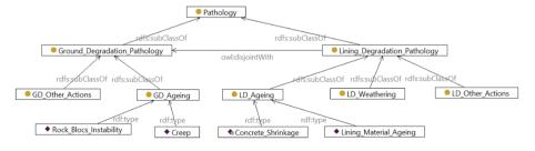
Fig. 5. Partial representation of pathologies classification based on degradation types.
