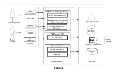
Fig. 1. PADTUN system architecture
