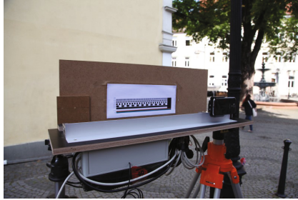
Fig. 5. (a) On site capturing setup: A tripod-mounted and battery-powered translation stage allows for horizontal camera shifts with welldefined velocities as well as for manual operation
