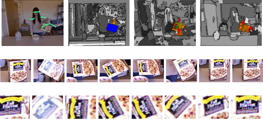
Fig. 2. Illustrating the tube generation process. The top row from left to right: The first image shows joint trajectories. The most active joint is used to compute the spatial prior for selecting superpixels. The three images next to it show three superpixel representations computed using depth (D), color (RGB) and both (RGBD). Colored superpixels are within the specified distance of the most active joint. Second and third rows visualize tubes T_v sampled from the blue and green superpixel S respectively.
