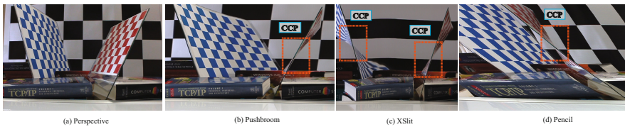
Fig. 7. Synthesized GLC images through stitching pinhole images. (a) The perspective view of the scene. (b) Pushbroom Image. (c) XSlit Image. (d) Pencil Image. Notice lines on a common 3D plane coverage t CCP in Pushbroom, XSlit and Pencil images.
