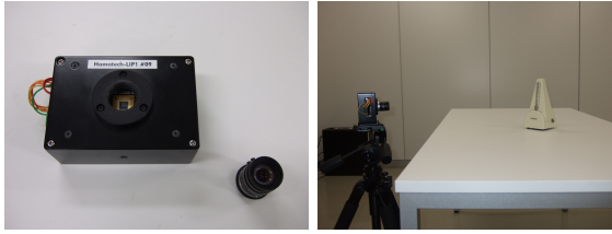
Fig. 6. A camera with the correlation image sensor (left) and the experimental setting (right)
