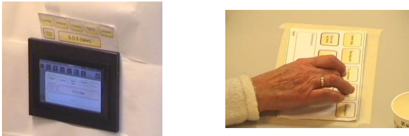
Fig. 2. An example of interactive prototype (left) and paper prototype (right) used in the usability experiment
