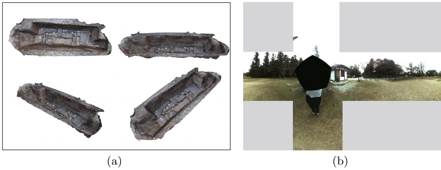
Fig. 3. Pre-collected data for creating cube environment map. (a) A 3D model of the ruin based on the measurement in multiple viewpoints. (b) A pre-captured panorama photo of the real environment.
