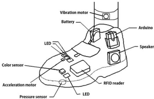
**Fig. 5.** System Configuration Design
