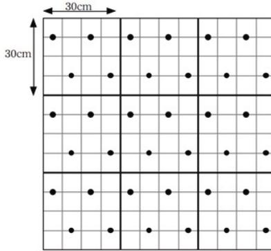
**Fig. 8.** Placement of RFID embedded to the ground Extracted from User location detection system using RFID[6]
