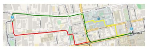
Fig. 3. Marking of routes (green: barrier-free, yellow: route includes surmountable barriers, red: route includes barriers)
