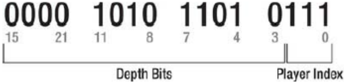
Fig. 5. Layout of the depth bits
