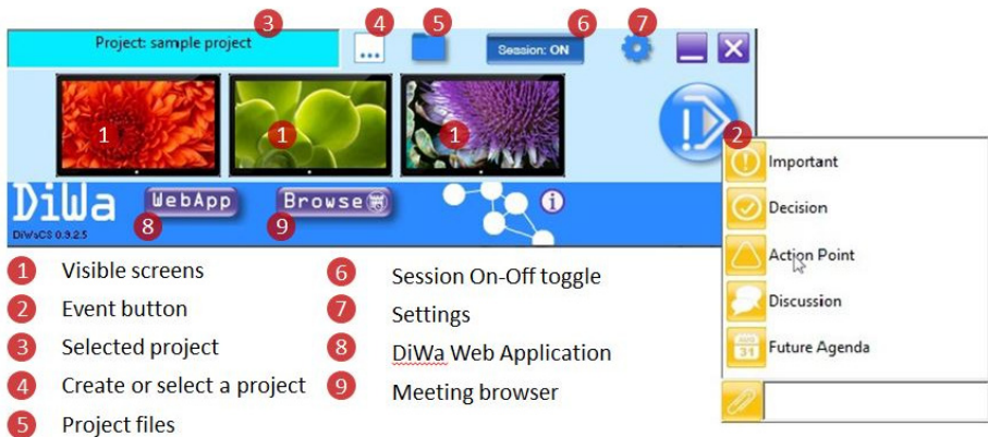
Fig. 2. The user interface of the DiWa Control Service with open event menu
