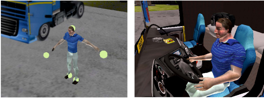
Fig. 1. Digital avatars represent specific personas. Mouse controls allow designers to control individual limbs using 'handles' and to automatically position personas, for instance on a seat in the cabin.
