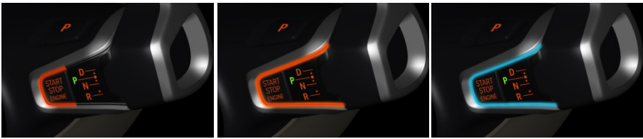
Fig. 6. Gear Shifter BMW i3 (Fotocredit: BMW Group): non-READY state (left), transition to READY state (middle), READY state (right). Night design, "P" active.
