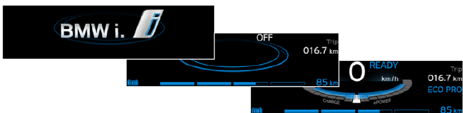
Fig. 5. Cluster Instrument BMW i3 (Fotocredit: BMW Group): Welcome (top), STAND BY (middle), READY (bottom)
