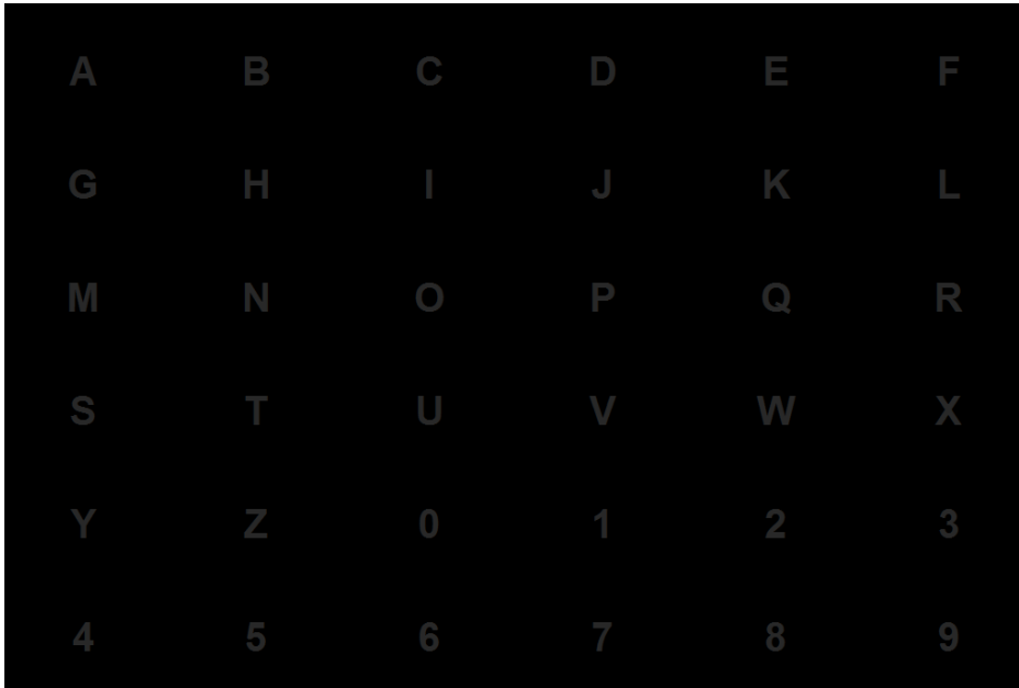
Fig. 3. The speller matrix consists of six rows and six columns leading to 36 characters in total
