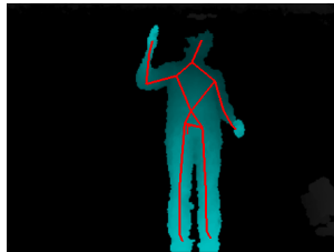
Fig. 2. The visualization of the depth map from Kinect by means of FFAST. The light blue area corresponds to the user, while the red lines indicate his simplified skeleton.
