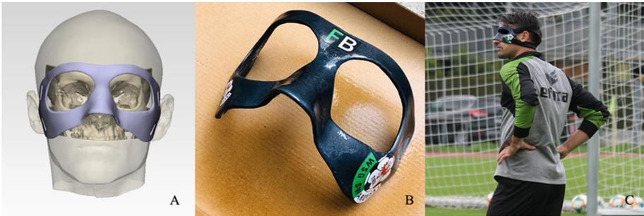
**Fig. 5.** Interactive digital workflow. A. 3D computer-aided design and planning B. FDM printed carbon-reinforced PLA face mask C. A professional soccer player with a customized face mask during his sport's practice session.
