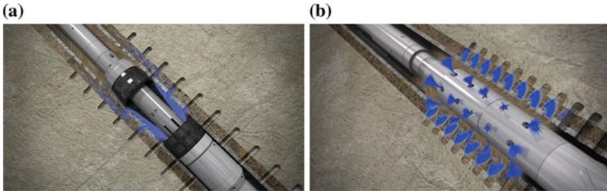
**Fig. 8.8** Washing tools for PWC technique; **a** swab cups create a seal inside casing and force the wash fluid into perforations, **b** jet tool sprays the wash fluid through perforations. (Courtesy of Hydrawell AS)
