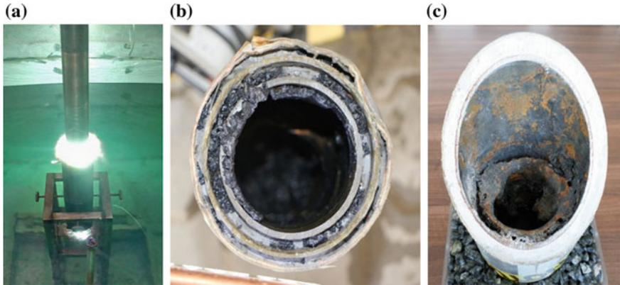
**Fig. 8.13** **a** Plasma-based tool entering a multistring casing sample; **b** upper view on the sample after the experiment; **c** sample after diagonal section in order to reveal obtained steel-cement removal [14]
