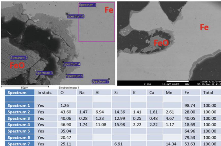
**Fig. 8.14** Samples of SEM image and EDX analysis of cuttings' material formed during plasma-based steel removal process of S355. (Courtesy of GA Drilling)
