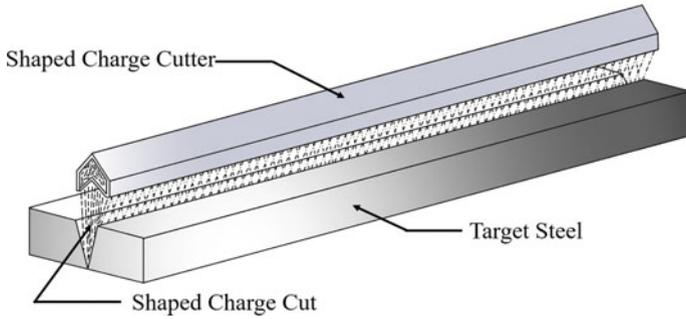
**Fig. 8.17** Drawing of a shaped charge cutter and the provided cut in the steel target [17]
