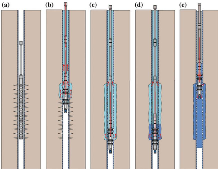
**Fig. 8.4** Perforate and wash part of PWC technique; **a** casing is perforated, **b** washing tool is RIH and washes the annular space behind the perforated interval, downward, **c** BHA is placed below the bottom perforations, **d** spacer is pumped and work string is pulled, upward, **e** spacer is extended above the top perforations. (Courtesy of Archer Oiltools)
