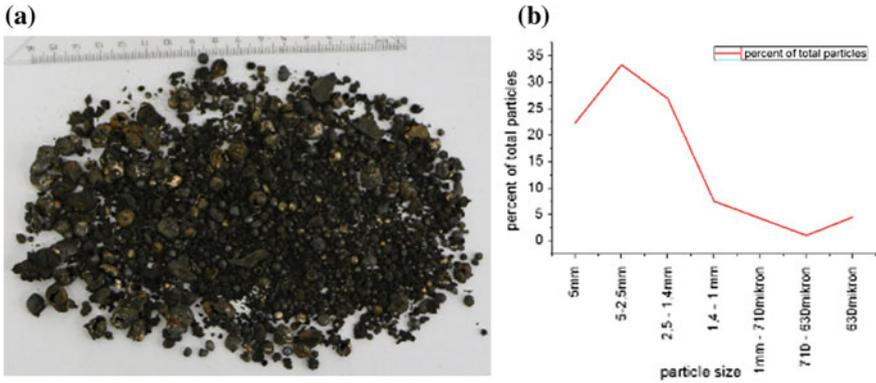
**Fig. 8.15** a Cuttings generated during plasma milling processes in water environment (scale in mm); b cuttings size distribution [16]
