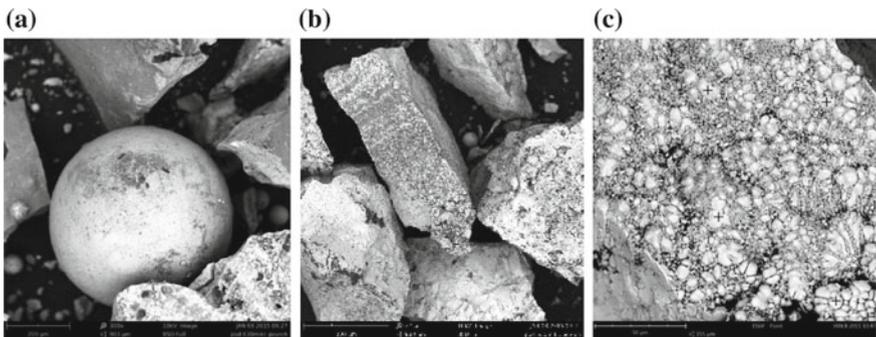
**Fig. 8.16** a Spherical cutting particle having ferritic structure; b and c SEM photo of oxidized cuttings surface. (Courtesy of GA Drilling)
