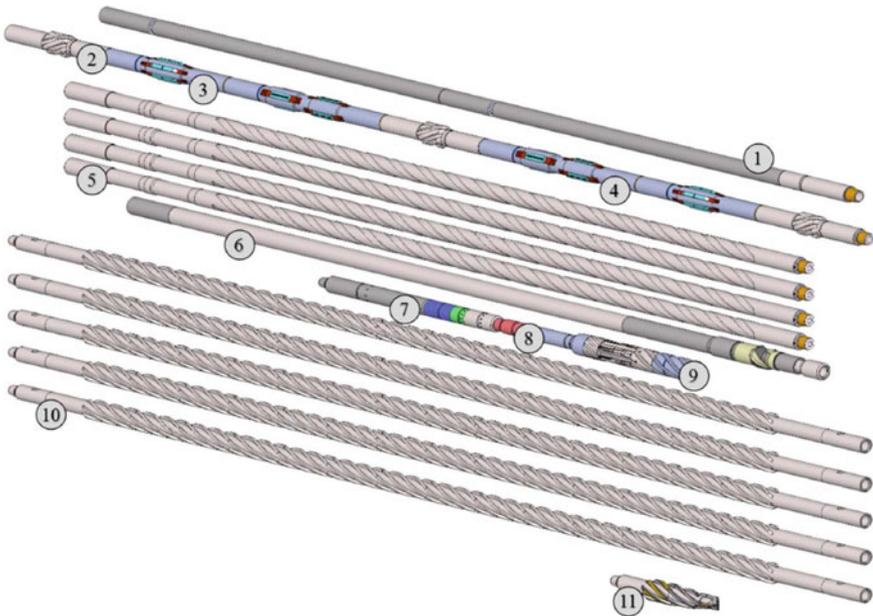
**Fig. 8.3** Main components of an upward milling BHA without swarf to surface; (1) intensifier, (2) spiral stabilizer, (3) spring loaded pads, (4) torque isolator, (5) drill collars, (6) left-hand mud motor (7) jet sub, (8) disconnect, (9) section mill, (10) auger section, and (11) taper mill [3]
