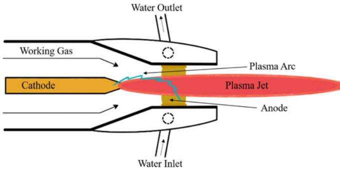
**Fig. 8.11** A non-transferred plasma cutter based on hot cathode
