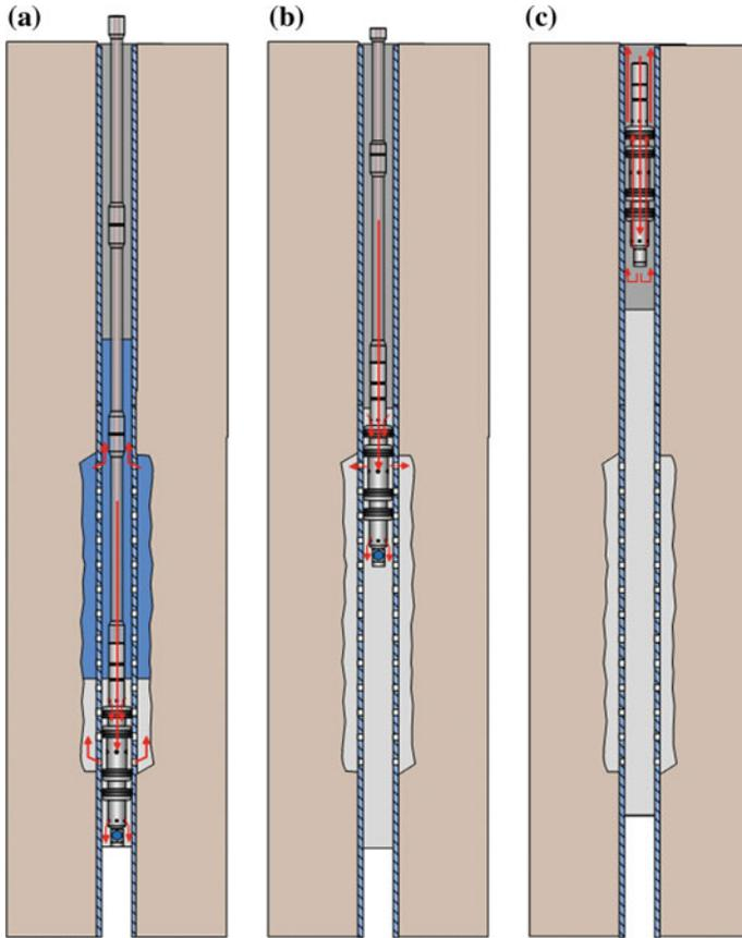
**Fig. 8.6** Cementing part of PWC technique; **a** BHA is placed below the bottom perforations, pumping few volumes of cement, **b** pump-and-pull while cementing, **c** pump cement and circulate out the cement in BHA, pull the BHA out of cement, at least 2 stands above top of cement. (Courtesy of Archer Oiltools)
