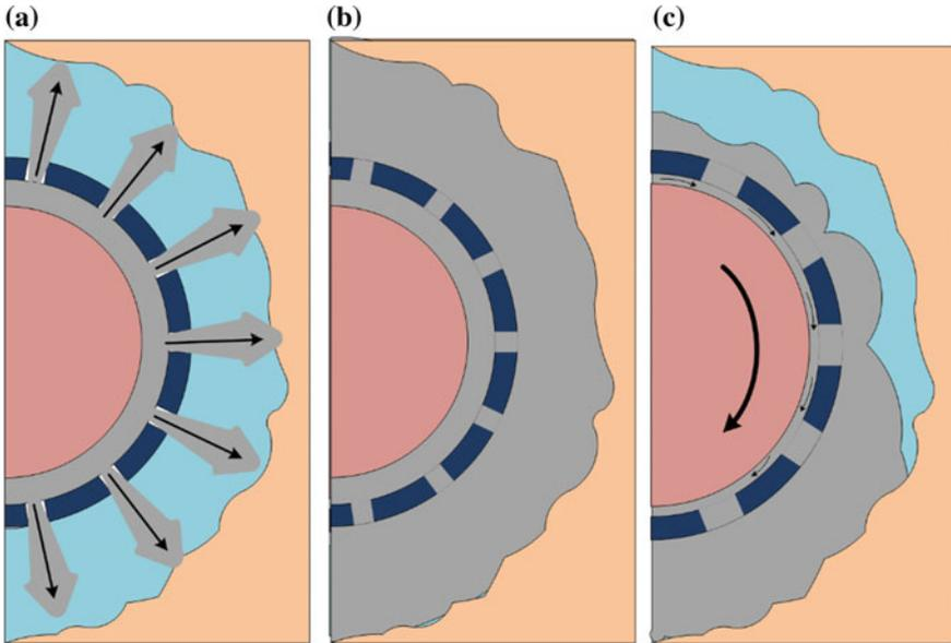
**Fig. 8.9** Cementing of perforated casing in PWC technique; **a** cement is pumped through perforations, **b** the ideal cement job to be expected, **c** due to inefficient displacement and inclination cement slurry may not be able to fully displace spacer
