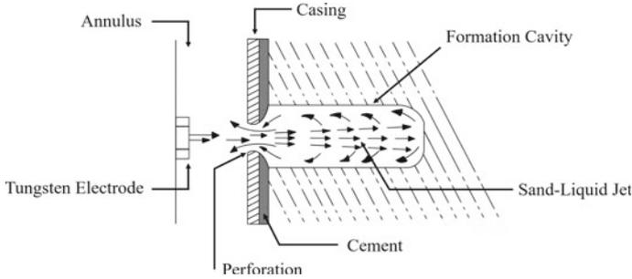
**Fig. 8.25** Abrasive cut process for a cemented casing
