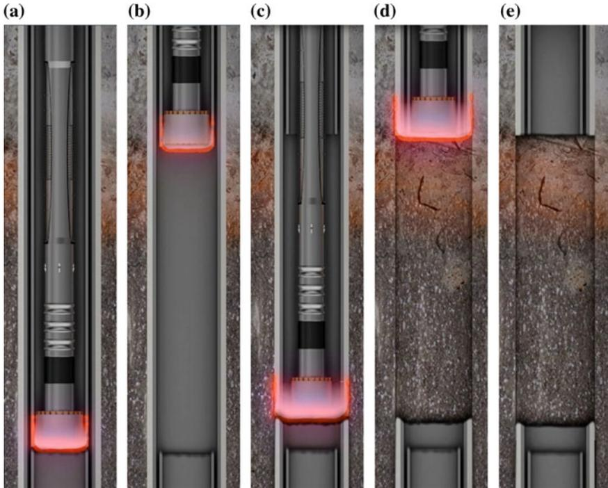
**Fig. 8.12** Casing section milling of tubing and casing with plasma-based tool. (Courtesy of GA Drilling)
