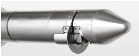
**Fig. 8.2** Mechanical pipe cutter which is powered hydraulically. (Courtesy of Schlumberger)
