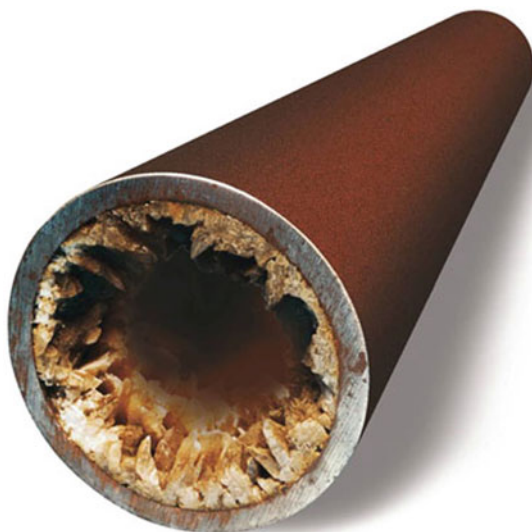
Fig. 2.8 Scale deposit caused a restricted access to downhole (Courtesy of Schlumberger)
