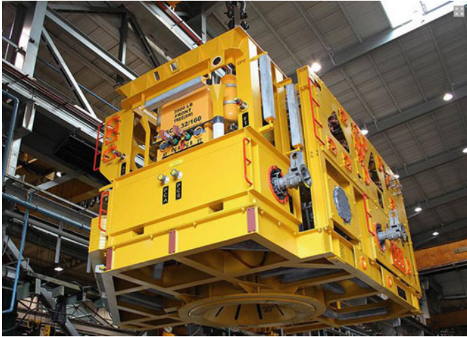
Fig. 2.20 A dual-bore vertical subsea tree which allows to monitor annulus pressure. (Courtesy of Schlumberger)
