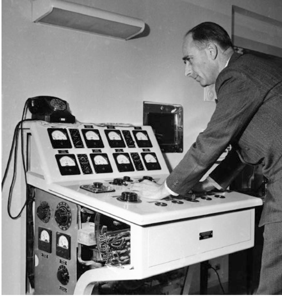
Rolf Widerøe at the control panel of the betatron that was developed for the Norwegian Radium Hospital, his second 31 MeV betatron, which was delivered in 1952. ( Photo NTB scanpix)
