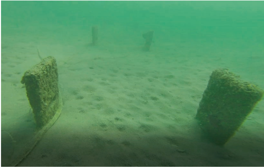
Fig. 10.4 Buried sleepers, 2 weeks after burial, showing endplates and slot (covered in growth) standing 50 cm apart above seabed
