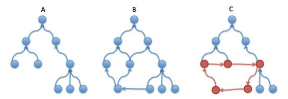
Fig. 1 (a) A simple hierarchical tree, (b) a directed, acyclic graph, (c) a graph that contains a cycle, indicated in red
