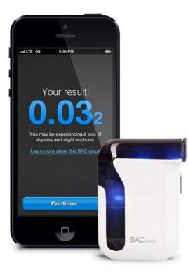
Figure 10-11. BACtrack Fuel Cell personal breathalyzer (image used with permission from BACtrack)
