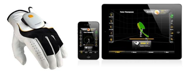
Figure 10-5. The GolfSense inertial sensor for golf swing analysis (image used with permission from Golfsense)
