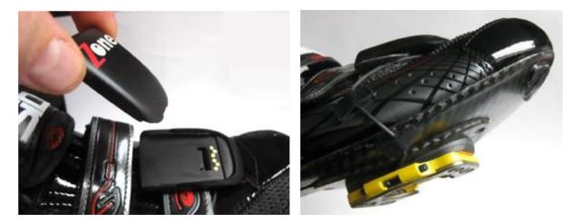
*Figure 10-4.* (a) Data collection pod, (b) strain gauge sensors attached to cleat (image used with permission from Brim Brothers)
