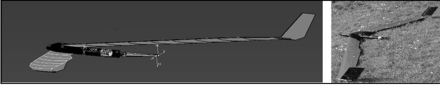
Figure 5 Carbon fibre reinforced flying wing with 2,6m wingspan
