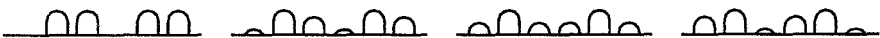
Fig. 2. 1 mm spaced pins displaying two braille dots moving laterally by steps of 0.25 mm
