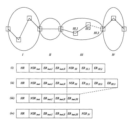
Figure 3. An establish\_request control message at various points along a path through networks *I*, *II*, *III*, and *IV*. Ellipses represent networks and squares represent nodes along the path. A node in two adjacent networks is a router, which considered to be a part of both networks.
