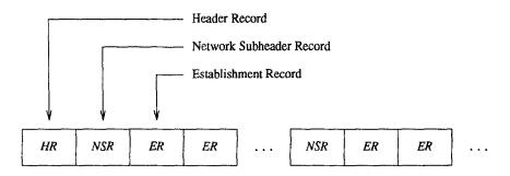
Figure 2. Structure of an establish\_request message. The start of the message is to the left. The Establishment Records (ERs) following a Network Subheader Record (NSR) contain establishment information on nodes within the network associated with the NSR.
