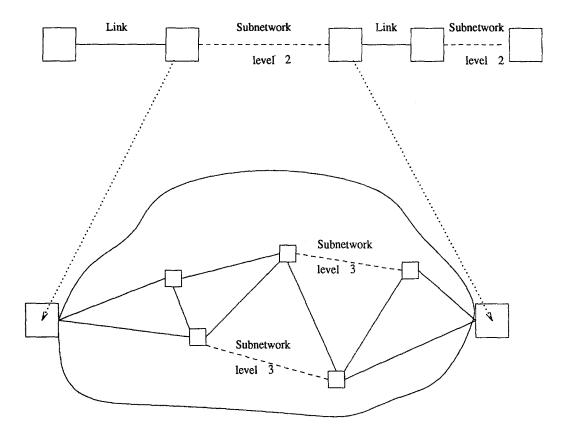
**Figure 1.** Hierarchic view of the internetwork. The network can be viewed as composed of nodes joined together by links which are either physical links or subnetworks.
