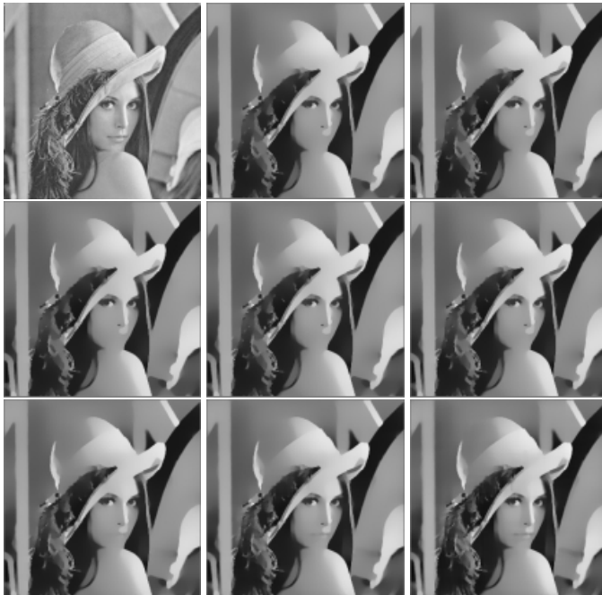
Fig. 1. Results of implicit difference scheme for Beltrami flow till scale = 250; the first row shows the initial image and results with f = 1, 2 ; second row corresponds to f = 5, 10, 20 ; third row corresponds to values of f = 50, 100, 200 .
