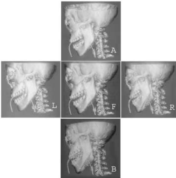
Fig. 3. Photos of projected stereoscopic skull images (stationary) by IV, taken from various directions. They show the motion parallax. The letter denotes the position of the observer to the IV stereoscopic image: A: above, L: left, F: front, R: right, B: below
