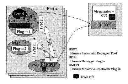
Fig. 2. Fundamental Architecture of Systematic Debugger In Harness
