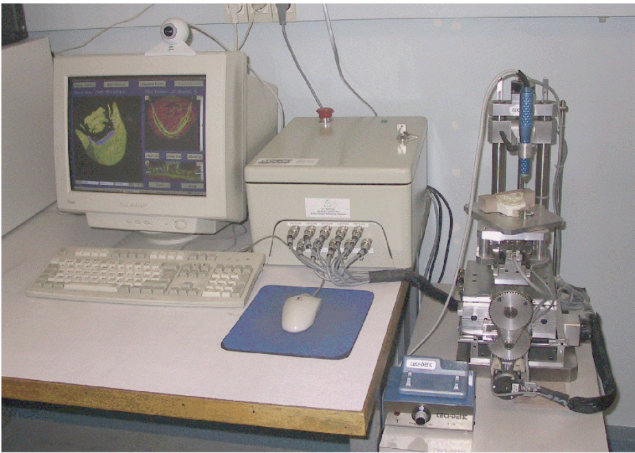
Fig. 3. Complete processing workbench, from pre-operative planning to splint drilling
