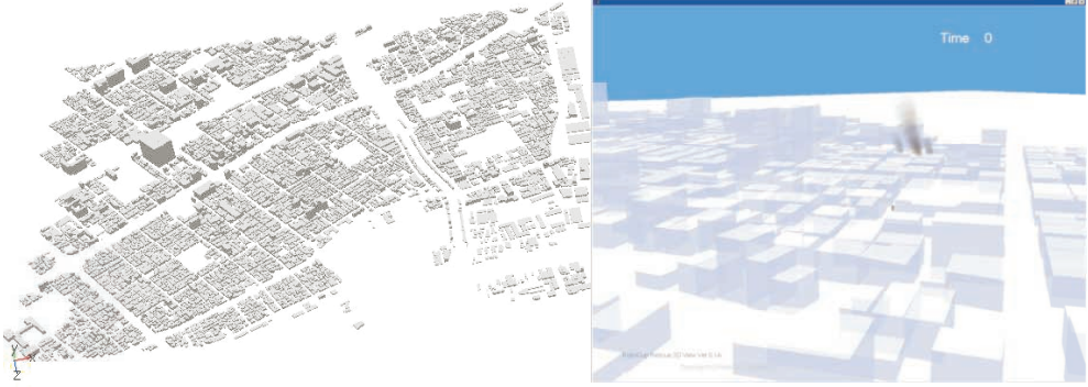
Fig. 2. Snapshot of a 3D data image of part of Nagata-Ward, Kobe(left) and a snapshot of 3D viewer(right) : The area shown is about 1.5 km by 1.5 km. As there are about 10,000 building in the area, the 3D viewer need to handle more than 50,000 polygons. Buildings are displayed as transparent objects in 3D viewer.
