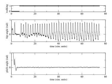
**Fig. 2.** Motion patterns of walking in the actuated biped robot. On top: the state of the waling behavior. Middle: Motion pattern of the left hip. The motion pattern is not entirely regular. Below: The state of the pitch value  $(\alpha)$ . A small oscillation is to see.
