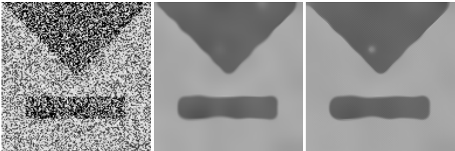
Fig. 3. Left to right: (a) Test image with noise. (b) Denoised by edge-enhancing diffusion with standard explicit scheme, \lambda = 5 , \sigma = 1.8 , \varrho = 0 , \tau = 0.166 , N = 200 iterations. (c) Denoised by edge-enhancing diffusion with LSAS, \lambda = 5 , \sigma = 1.8 , \varrho = 0 , \tau = 1 , N = 200 iterations.
