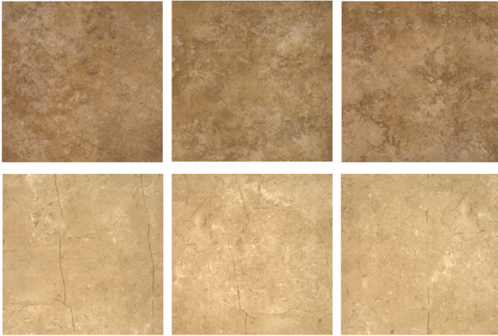
Fig. 2. Samples from the ground truth. From up to down; three samples of petra and marfil models, each one corresponding to a different surface grade.
